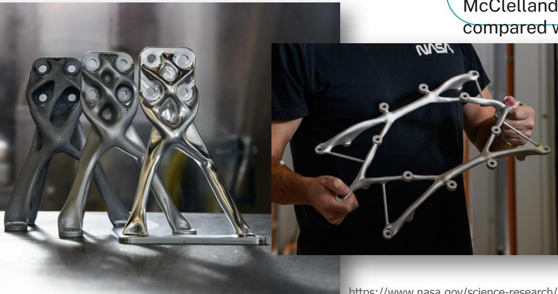
“These evolved structures save up to two-thirds of the weight compared to traditional components, he said, and can be milled by commercial vendors. “You can perform the design, analysis and fabrication of a prototype part, and have it in hand in as little as one week.”
